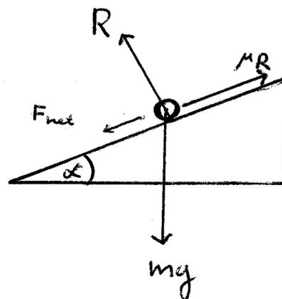
The only difference to the above calculation for the particle being projected up the plane is the reversal of  $F_{\text{net}}$  and  $\mu R$ . This leads to
