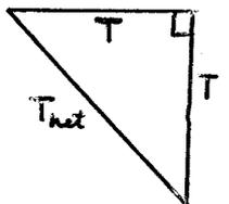
$$T_{net}^2 = T^2 + T^2 \Rightarrow \underline{T_{net} = \sqrt{2} \left( \frac{Mm}{M+m} \right) g}$$
